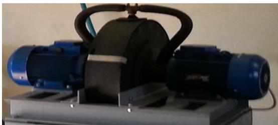
Figure 2: General view of the experimental hydrodynamic activator
