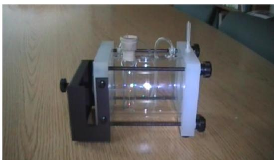
Figure 1: Electrochemical three electrode flat cell kit (K0235).
