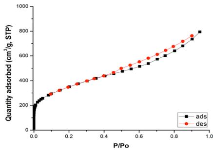
**Fig. 1.** Isotherm of low-temperature adsorption of nitrogen for active carbon derived on the basis of rice husk
