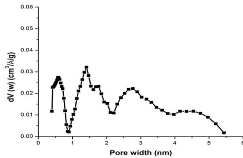
**Fig. 2.** Pore size distribution of active carbon derived on the basis of rice husk
