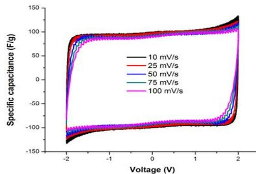
**Figure 4** – Effect of scan rate on charge propagation and capacitance of composite electrodes with EMITFSI
