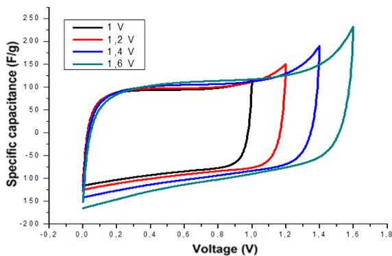
**Figure 3** – Effect of voltage limits on cyclic voltammograms of composite electrodes with 1M  $\text{Li}_2\text{SO}_4$
