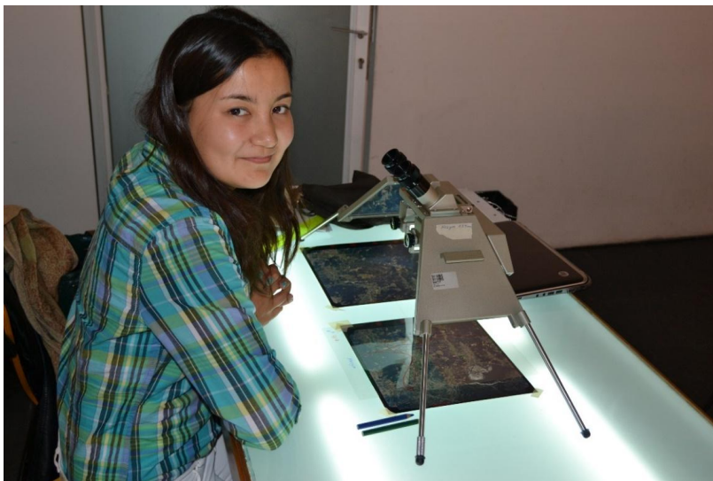
Fig.5 Stereoscope - an instrument that lets an operator see two photos at once in a stereo view
