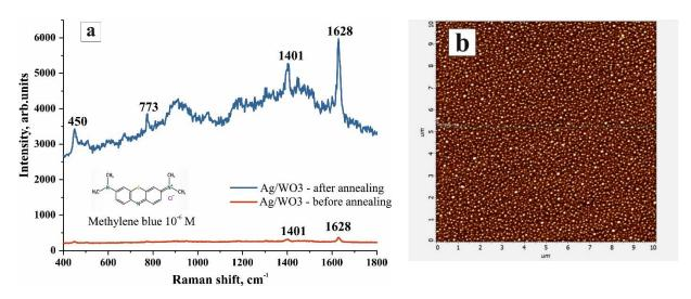
Fig. 1. – Raman spectrum of Methylene blue 10<sup>-6</sup> M (a) and AFM image of Ag NPs/WO<sub>3</sub> after annealing (b)
