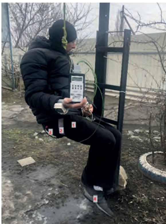
Figure 1. Points of locations of temperature sensors: sensor No. 1 (on the surface of the hip), sensor No. 2 (on the body surface under the safety system belt), sensor No. 3 on the body surface in the buttock area, sensor No. 4 (on the foot surface) in shoes
