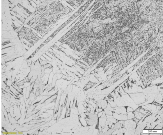
Fig. 3. Signs of uneven cooling, *100
