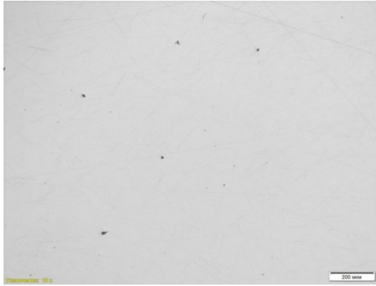
Fig. 7. Single non-metallic inclusions, *100
