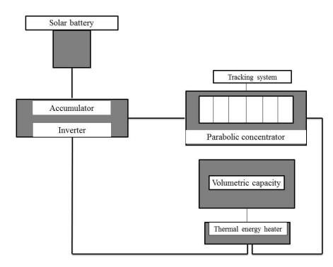
Figure 2. Schematic diagram of solar device equipped with concentrating elements
