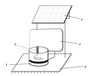
1 - a cylindrical container, 2 - copper tube, 3-cell battery, 4 - parabolic concentrator, 5 - base made of steel;
