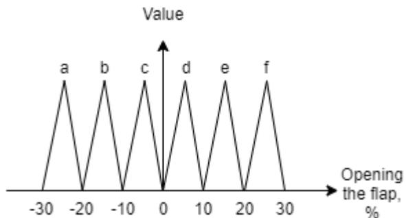
Fig. 6. Graphs of membership functions for the term of the linguistic variable "percentage of opening of the VL flap": a-open a lot; b-open an average; c-open a little; d-close a little; e-close an average; f-close a lot
