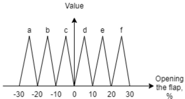
Fig. 5. Graphs of membership functions for the term of the linguistic variable "percentage of opening the flap DRY": a-open a lot; b-open average; c-open little; d-close little; e-close average; f-close a lot
