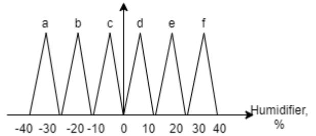
Fig. 7. Graphs of membership functions for the term of the linguistic variable "percentage of humidifier/dehumidifier inclusion": a-reduce a lot; b-decrease average; c-decrease a little; d-add a little; e-add medium; f-add a lot
