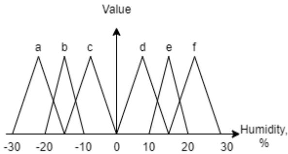
Fig. 3. Graphs of membership functions for the term of the linguistic variable "change in humidity in the room": a-large decrease; b-average decrease; c-small decrease; d-small increase; e-average increase; f-large increase
