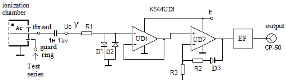
**Figure 2.** A schematic block diagram of the logarithmic amplifier of an IC recording channel.
