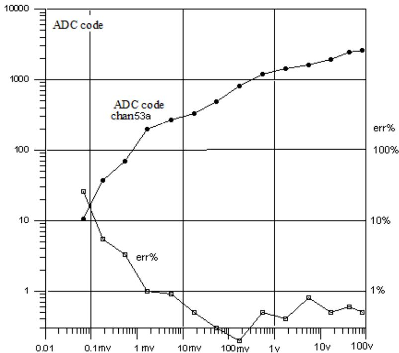
**Figure 3.** Transfer function of the amplifier of ionization chamber.
