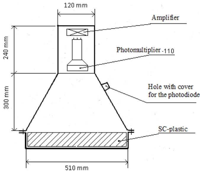
**Figure 4.** The design of the scintillation detector.
