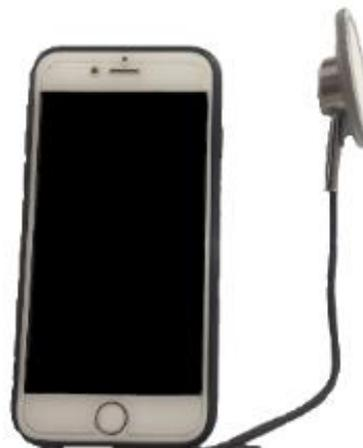
Fig. 4. Smart stethoscope as a device that connected to a smartphone
