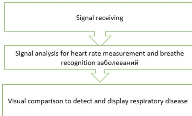
Fig. 2. Working principle of the smart stethoscope
