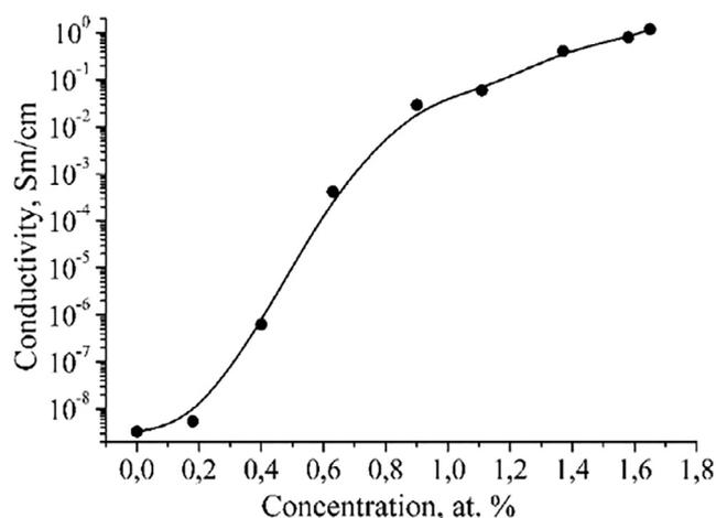
Fig. 6. The dependence of the conductivity on the Ir content in a-C <Ir> films at 300 K.
