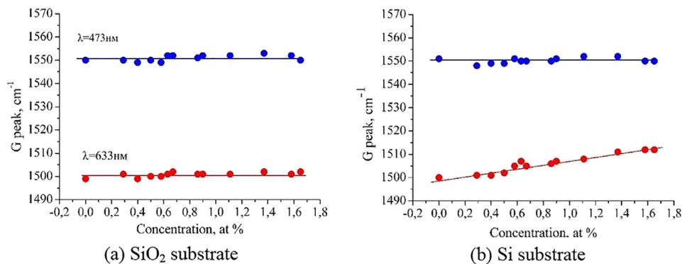
Fig. 3. The dependence of the G peak position on the Ir concentration in a-C films.
