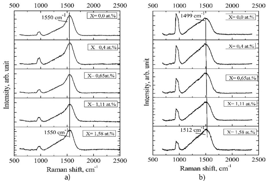
Fig. 2. Raman spectra a-C<Ir> films synthesized on a silicon substrate at excitation wavelength (a) 473 nm, (b) 633 nm.
