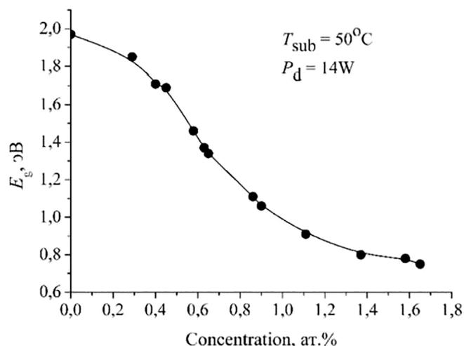
Fig. 5. Dependence of the optical band gap on the concentration of Ir.
