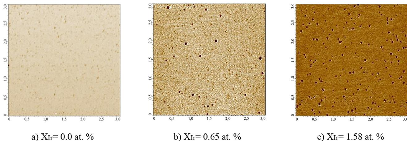
Fig. 1. Phase contrast AFM imaging of the surface of a-C <Ir<sub>x</sub>
