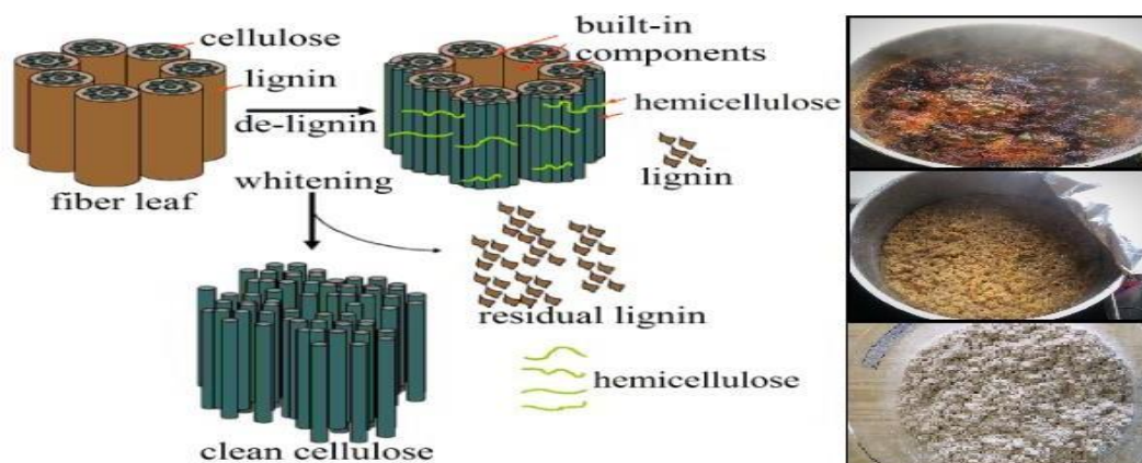
Fig.1. The main processes for boiling isolation of cellulose
