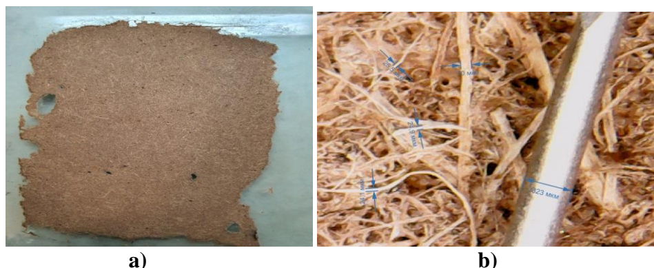
Fig.3. – a) Carton board; b) Optical microscope pictures (200x)
