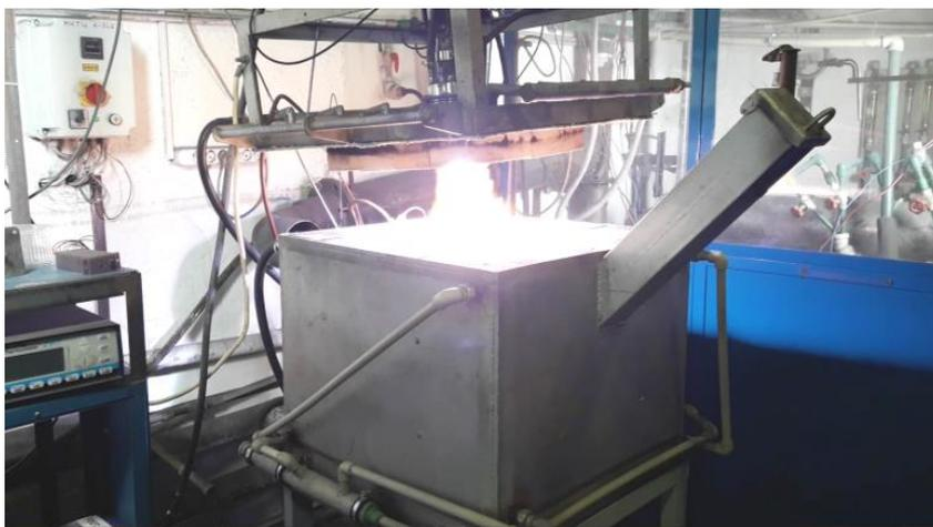
Figure 5. Photo of the plasma torch in action with lifted lid of the reactor.
