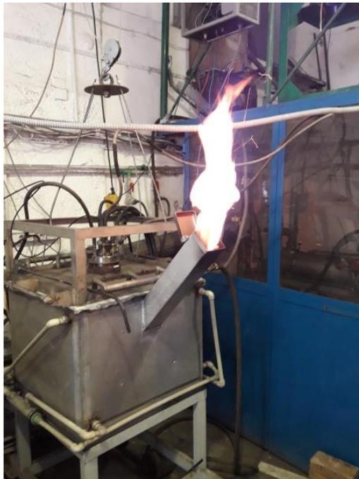
Figure 6. Photo of the combustible gas control flame from the pipe for supplying of briquetted WW.
