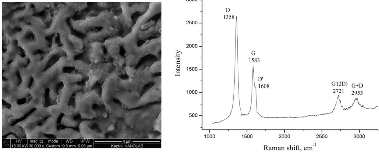
Fig. 6. SEM image and Raman spectrum of CNWs/Cu sample after PECVD synthesis.
