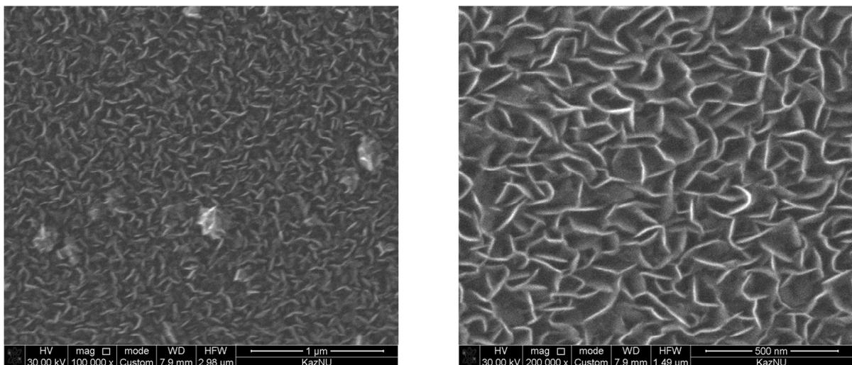
Fig. 3. SEM images of CNWs synthesized on Ni/Si substrate at RF power of 15 W.
