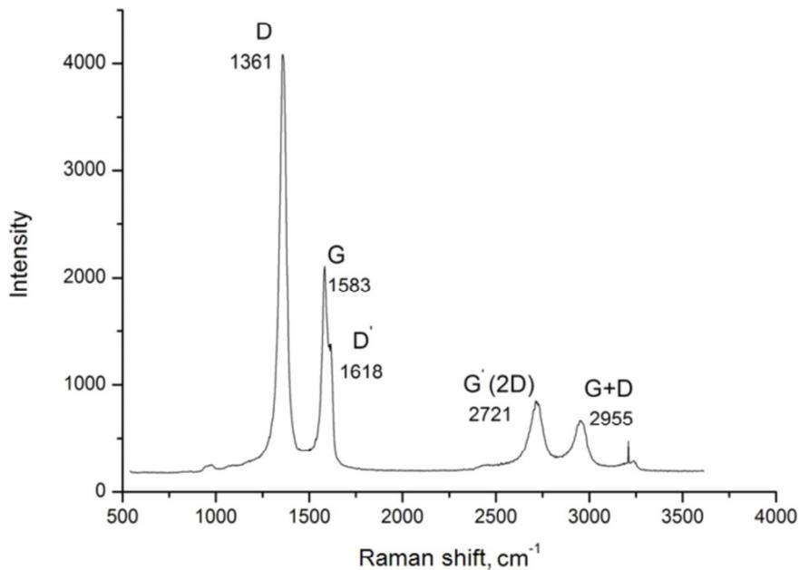
Fig. 5. Raman spectrum of CNW synthesized on Ni/Si substrate at RF power 15 W.
