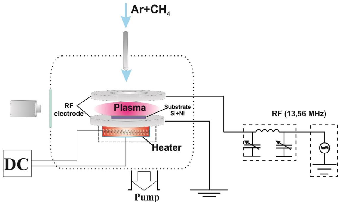
Fig. 1. Experimental setup for CNWs synthesis.
