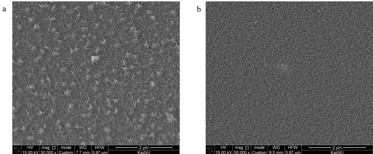
Fig. 2. SEM images of CNWs synthesized on Ni/Si substrates at RF powers of 15 W (a) and 10 W (b).
