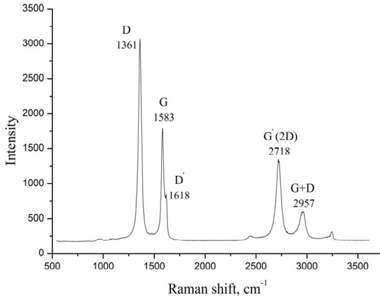
Fig. 4. Raman spectrum of CNW synthesized on Ni/Si substrate at RF power 10 W.
