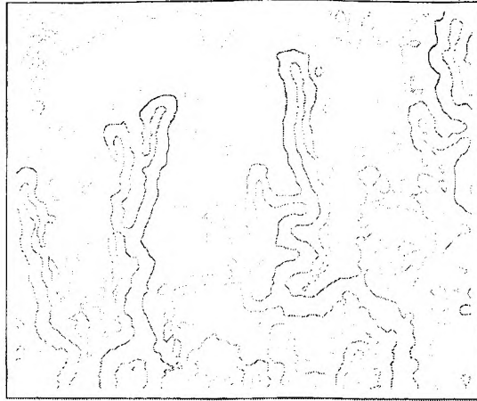
Figure 10. Resulting edge lines obtained by the method, based on finding intersection points of the boundary curves of the initial image and the sharpened image.
