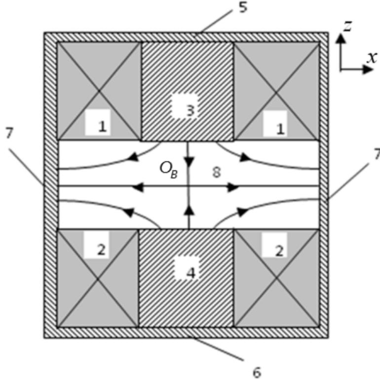
Figure 1: Sketch of the experimental setup creating a cusp magnetic trap. 1 and 2, solenoid coils; 3 and 4, cores of the coils (steel); 5 and 6, end magnetic conductors (steel); 7, side magnetic conductors; 8, working region is the magnetic trap. The case of identical currents in the coils  $i_1 = i_2$  is shown; point  $O_B$  is the magnetic well,  $\mathbf{B}(O_B) = 0$ . The arrows indicate the direction of the magnetic field lines.
