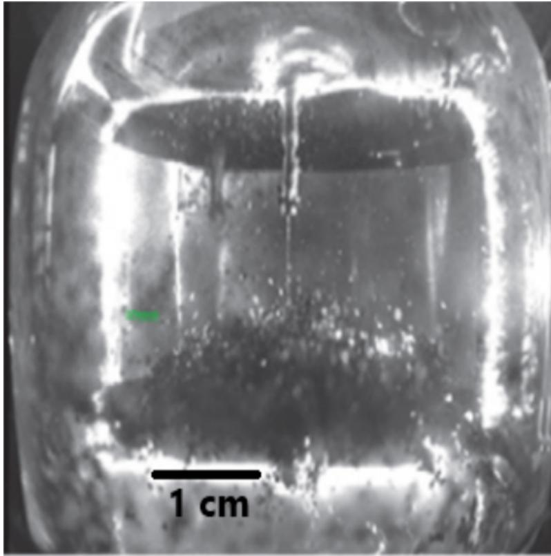
Figure 2: Initial position and shape of the cluster consisting of near 30000 initially uncharged graphite particles in the cusp magnetic trap at  $i_1 = 0.5i_m$  and  $i_2 = 0.3i_m$ .
