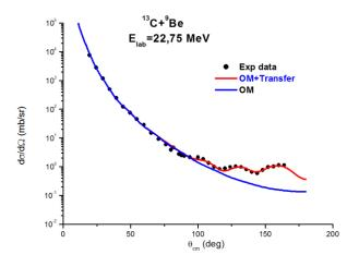
**Figure:** Angular distribution of the elastic scattering of <sup>13</sup>C on <sup>9</sup>Be at the  $E_{lab}$ =22.75 MeV. Circles are experimental data; the blue line is the optical model prediction, and the red line represents the coupled reaction channels calculation by code FRESCO with taking into account the exchange mechanism of the  $\alpha$ -cluster transfer.
