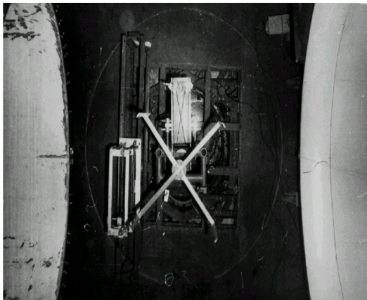
Figure 15. The active laboratory model of the Bi-Darrieus turbine in a working site of a wind tunnel (top view)
