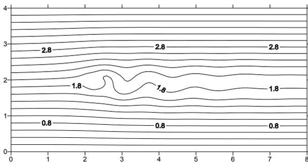
Fig. 11. Flow around a vertical rotating shaft
