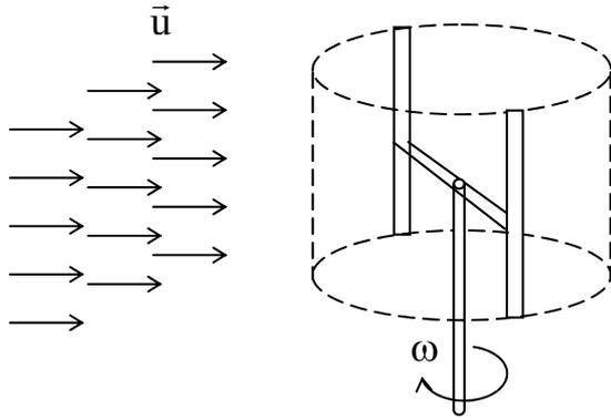
**Fig. 1.** Schematic of the wind turbine carousel
