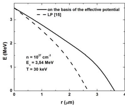
**Fig. 6.** The slowing down energy of the  $\alpha$ -particles with an initial energy  $E_0 = 3.54$  MeV.
