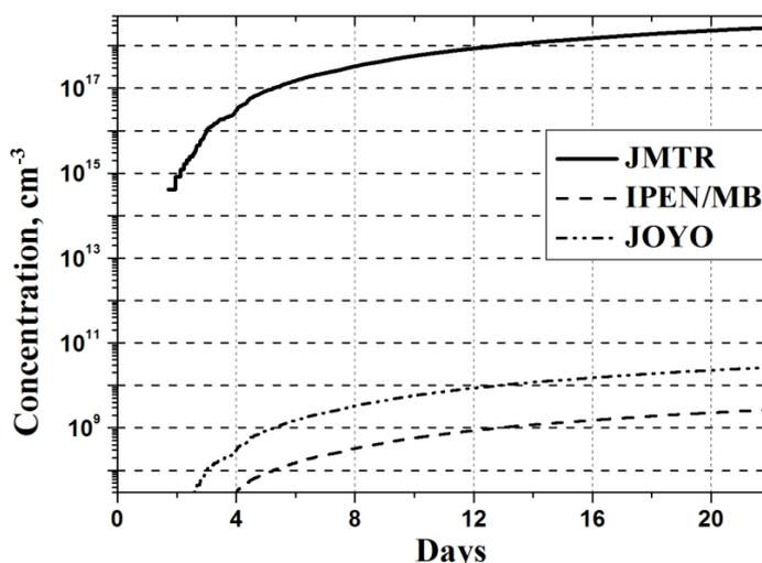
**Figure 4.** Here is shown the concentration of tritium in the Be<sup>9</sup> slab depending on time for spectrum of reactors JMTR, IPEN/MB and JOYO.
