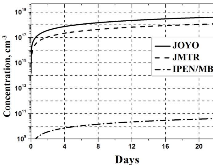
**Figure 5.** Here is shown the concentration of He<sup>4</sup> in the Be<sup>9</sup> slab depending on time for spectrum of reactors JMTR, IPEN/MB and JOYO.
