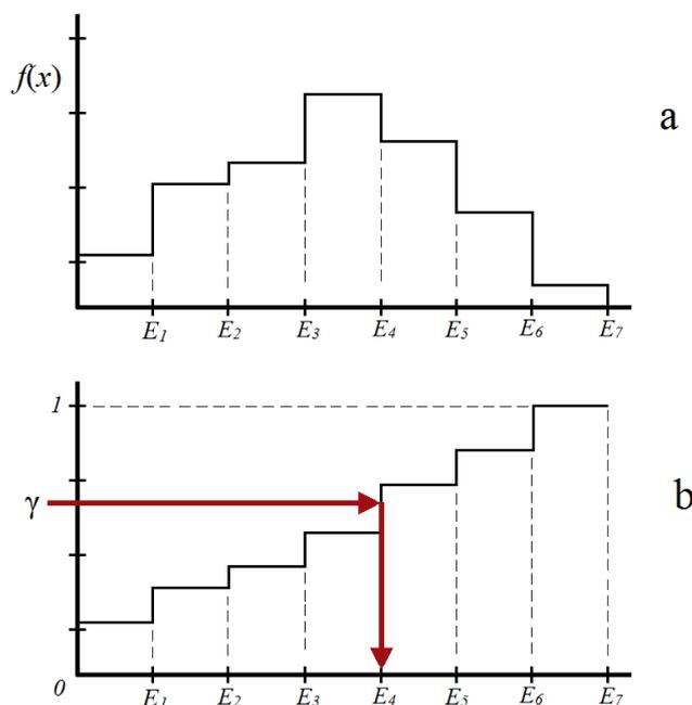
**Figure 2.** The scheme of selecting the initial energy of neutrons from neutron spectrum. The figure (a) shows neutron spectrum and figure (b) shows the stairs of probabilities.
