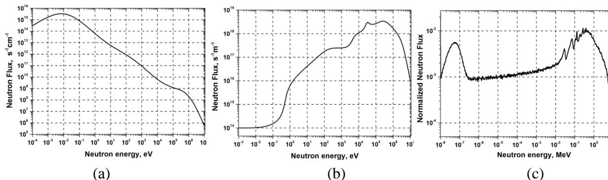
**Figure 3.** The neutron spectrums of the reactors IPEN/MB-01 (a), JOYO (b) and JMTR (c).
