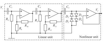
Fig. 3. Phase-shifting unit consists of two linear and one nonlinear shifting subunits.
