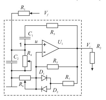
Fig. 2. Wien bridge oscillator. Here  $V_i$  is the output voltage of the *i*-th oscillator,  $V_f$  is the output voltage of the global feedback loop.
