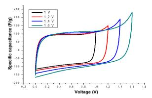
Figure 3 – Effect of voltage limits on cyclic voltammograms of composite electrodes with  $1M Li_2SO_4$
