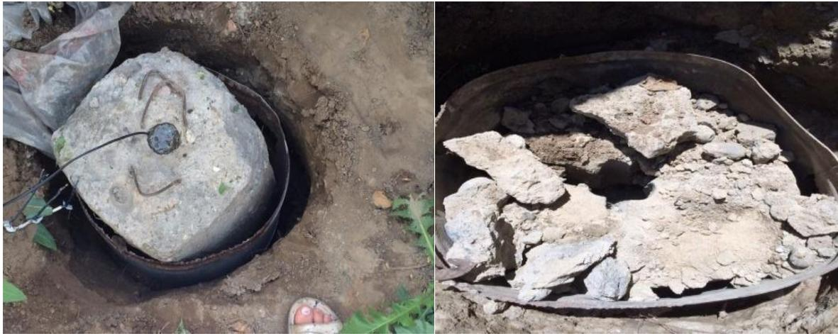
a) Monolithic concrete block, b) Monolithic concrete block is crushed by gas generator.
