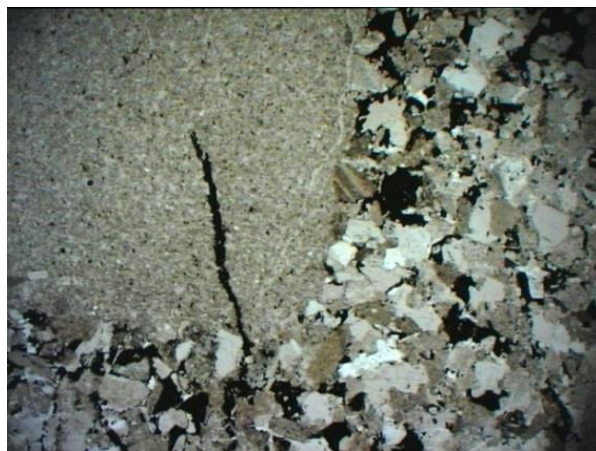
Figure 7: Image of aleurolite included in sandstone in the polarizing microscope in transmission light, power 25 x , without analyser
