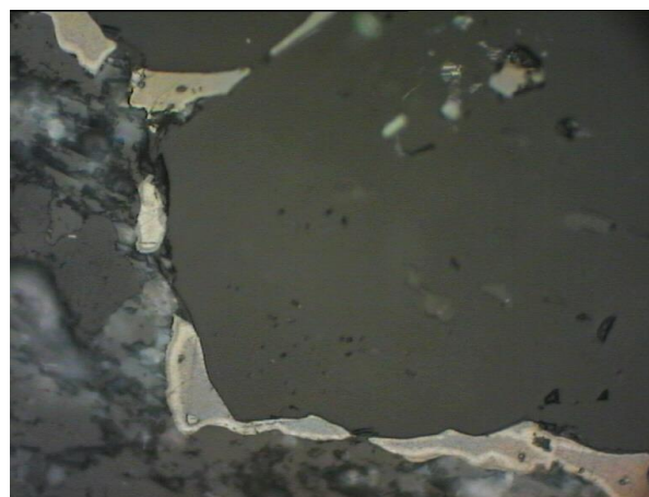
Figure 12: Image of pore cementation, chalcocite around quartz, in the polarizing microscope in reflection light, power 50^x , without analyser
