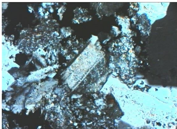
Figure 6: Image of sandstone in the polarizing microscope in transmission light, power 20 x , with analyser
