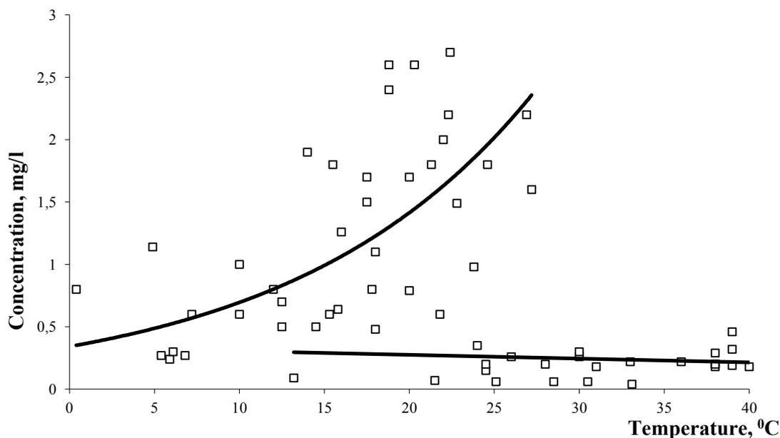
Figure 1 - The dependence of the oil content in the water on temperature of cooling reservoir Ekibastuz Power Plant-1
