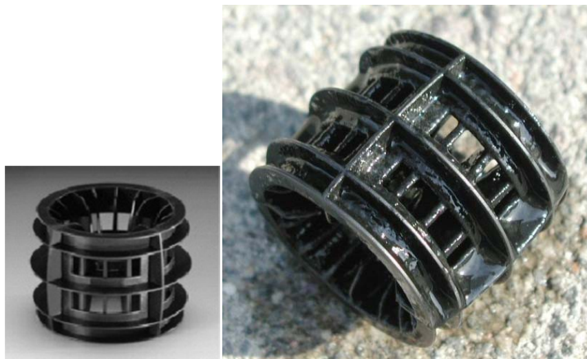
Fig. 4: Packing material without (left) and with immobilized biofilm
