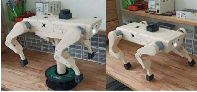
Fig. 6. Prototype of the robot made with 3D printing
