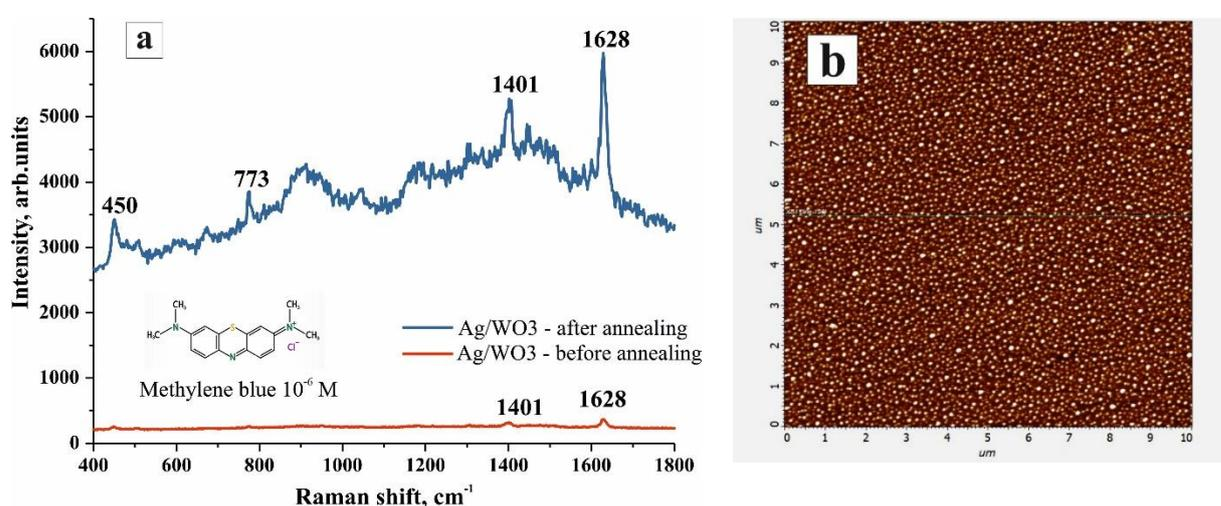
Fig. 1. – Raman spectrum of Methylene blue 10<sup>-6</sup> M (a) and AFM image of Ag NPs/WO<sub>3</sub> after annealing (b)
