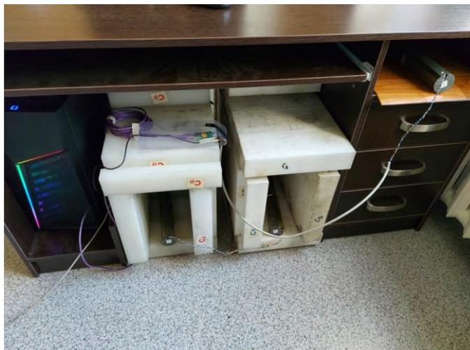
Figure 1 - The view of the detectors and their polyethylene and borated polyethylene coverings
