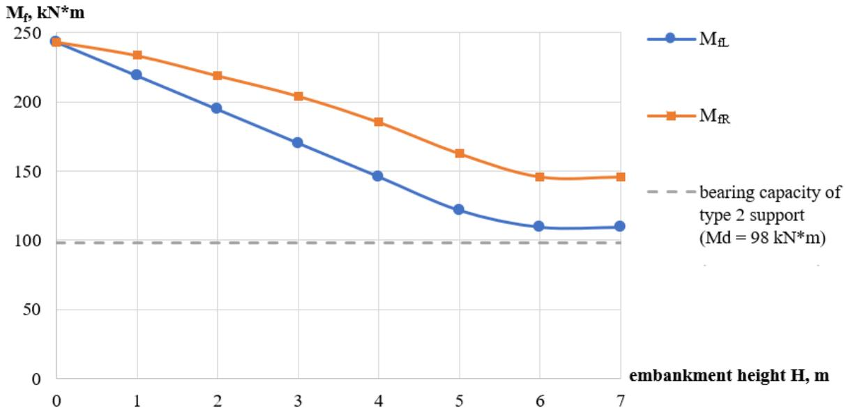
Fig. 3. Graph of change in bearing capacity of 8 m long pile foundation on sandy soil subgrade
