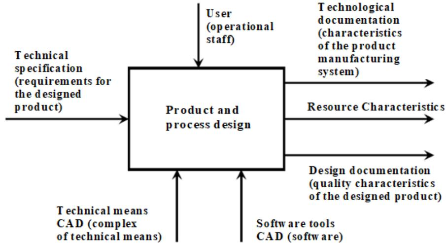
Fig. 3. General scheme of the process of designing and developing a product using CAD tools
