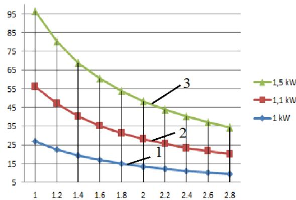
Fig. 2. Dependence of the rotational force values generated at the surface points of the wheel on the power of the driver and the speed of rotation of the wheel
