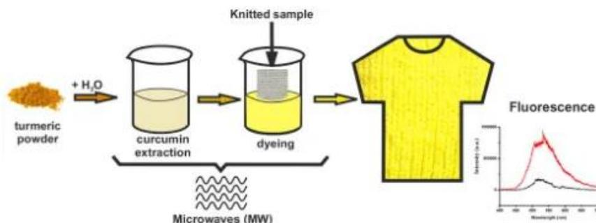
Fig.5. Dyeing using Microwave Technology.
