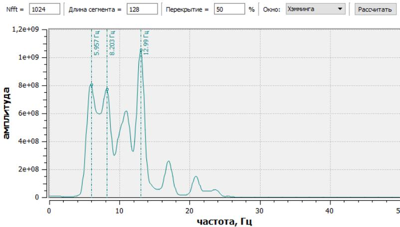
Fig. 9. Vibration frequency spectrum of superstructure No. 1 (left)
