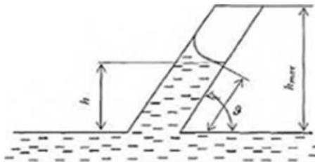
Fig. 4. The height of the liquid rise in an inclined cylindrical capillary
