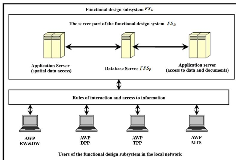
Fig. 5. Organizational scheme of the functional subsystem of the design of the FPS\_PR products
