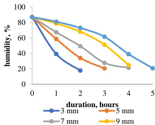
Fig. 9. Curves for combined infrared and convective drying at temperature 60 °C of apple slices treated by salt solution
