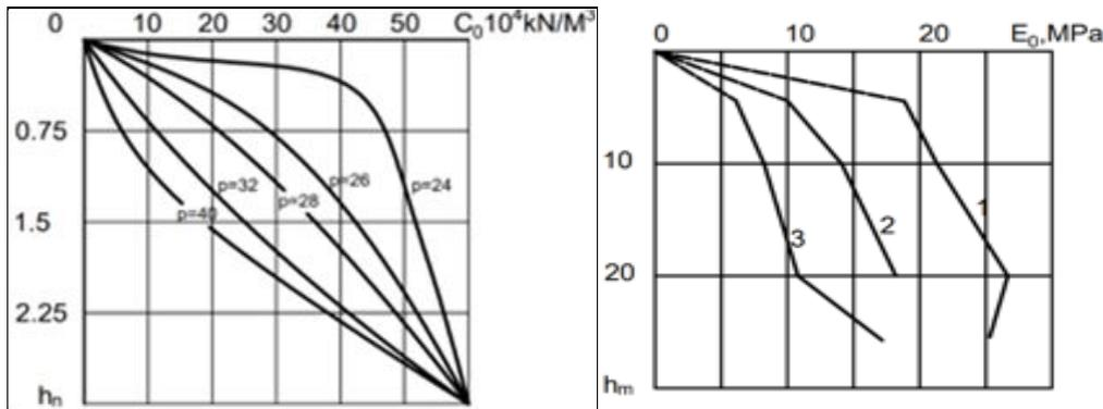
Fig.1. (a) The depth deformation modules of the soil at natural (1), soaked (2) and desalinated (3) and the nature of the distribution of the stiffness coefficient  $C(x_k)$  in depth depending on the steps of the applied forces (for example, Central Fergana).
