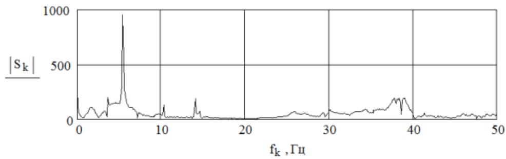
Fig. 4. Spectrum of vibration displacement of the superstructure of a metal bridge, seismic receiver №1, maximum spectral surge at a frequency of 5.47 Hz
