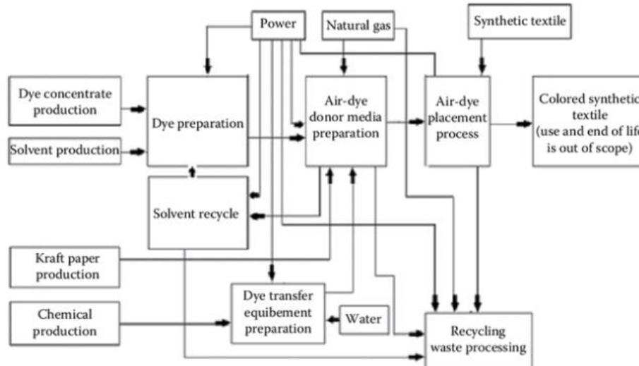
Fig. 7. Flow chart of Air-dye technology.
