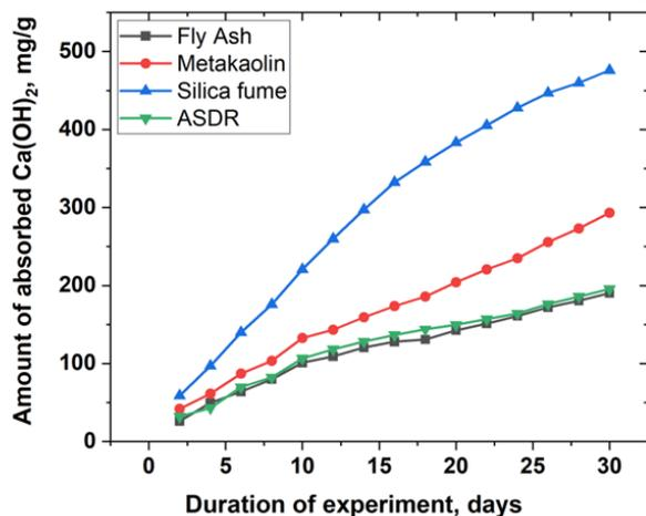
Fig.3. Absorption by mineral additives of Ca(OH)<sub>2</sub> in time, from saturated lime solution
