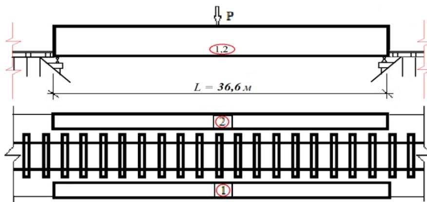
1 and 2 – seismometers installed in the middle of the span;  $P$  – load from one person (impulse – jumping)
