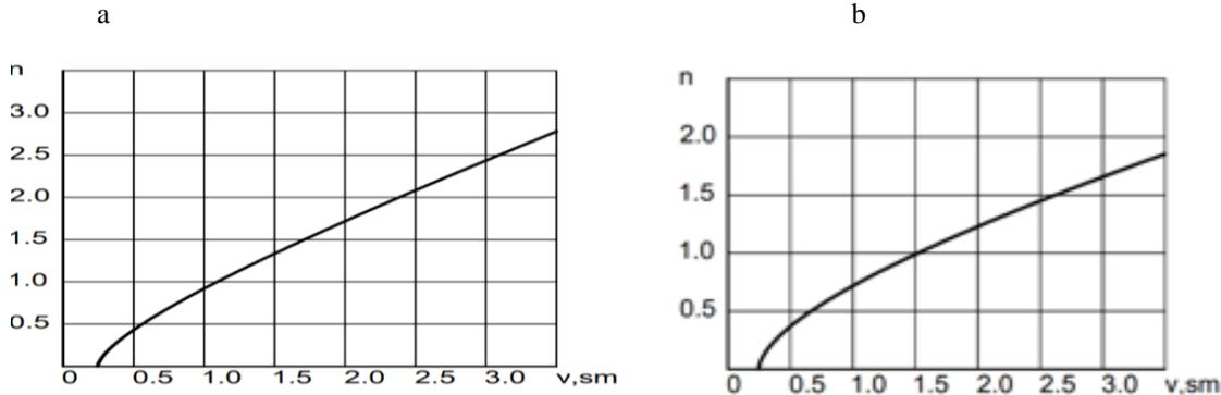
Fig.2. Parameter  $n$  for flexible (a) and rigid (b) piles.
