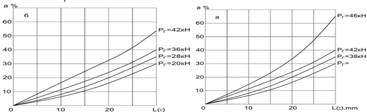
Fig.4. The effect of the predicted depth of concrete corrosion on the horizontal movements of the pile head at different ground conditions: *a*-  $C_o = 7,9 \cdot 10^4 \text{ kN/m}^3$ ; *б*-  $C_o = 6 \cdot 10^4 \text{ kN/m}^3$ .
