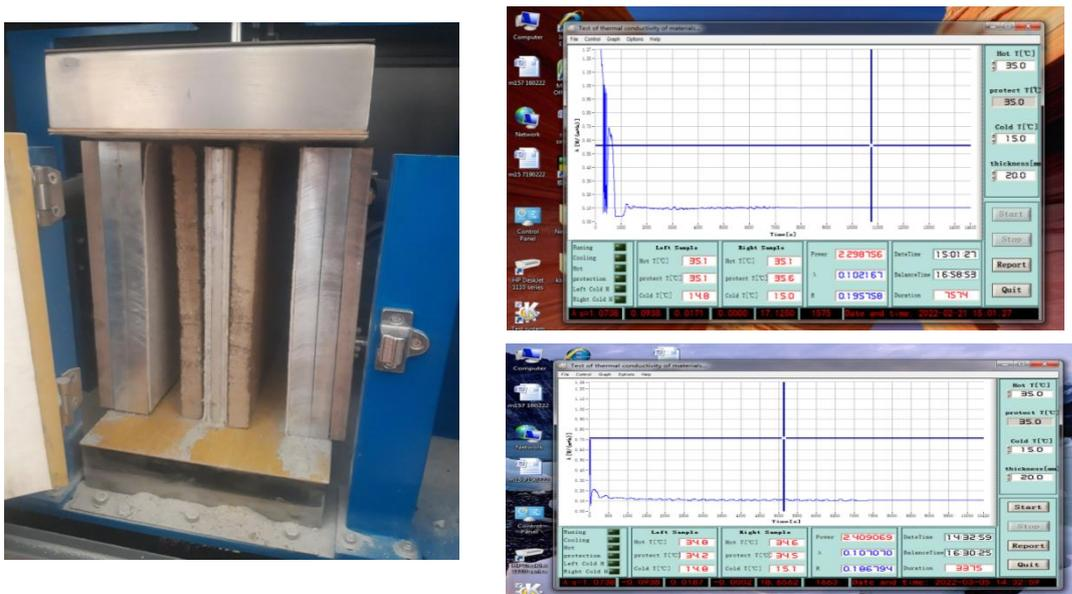
Fig.2. ((XD-2-30C machine) Determination of heat transfer coefficient of vermiculite plate
