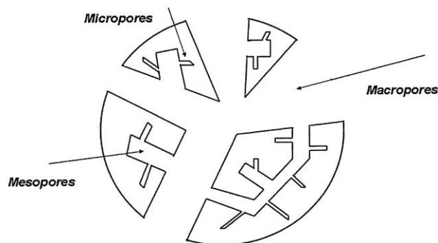
Fig.1. Pore structure of activated carbon
