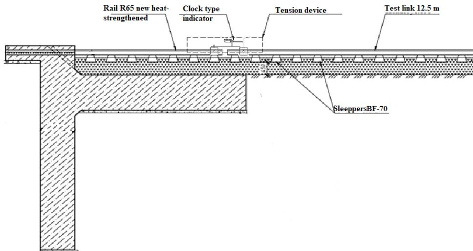
Fig. 1. Test bench for determining linear resistance to longitudinal movement of rails on sleepers.
