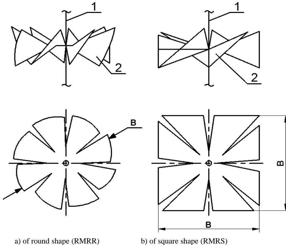
Fig. 1 - Designs of rotating plate packing elements.
