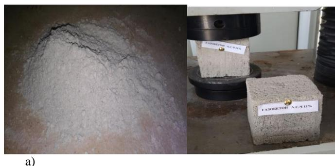
Fig-1. a) asbestos cement. b) aerated concrete
