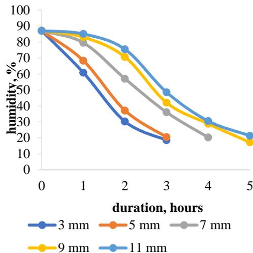
Fig. 5. Curves for combined infrared and convective drying at temperature 55 °C of apple slices treated by salt solution
