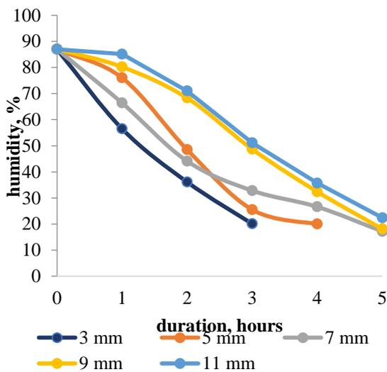
Fig. 2. Curves for combined infrared and convective drying at temperature 55 °C of control samples of apple slices
