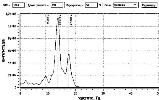
Fig. 6 Vibration frequency spectrum of superstructure No. 1
