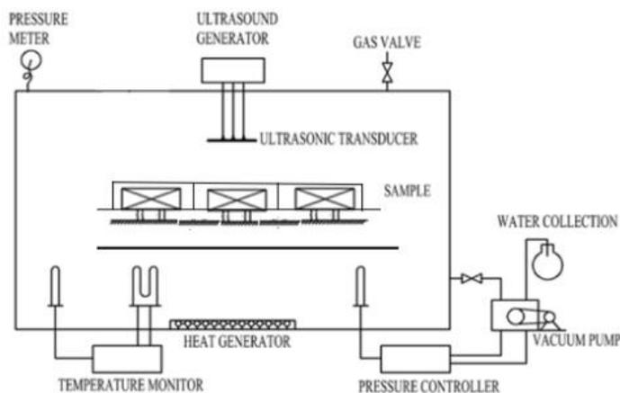
Fig. 6. Ultrasonic Wave Dyeing.
