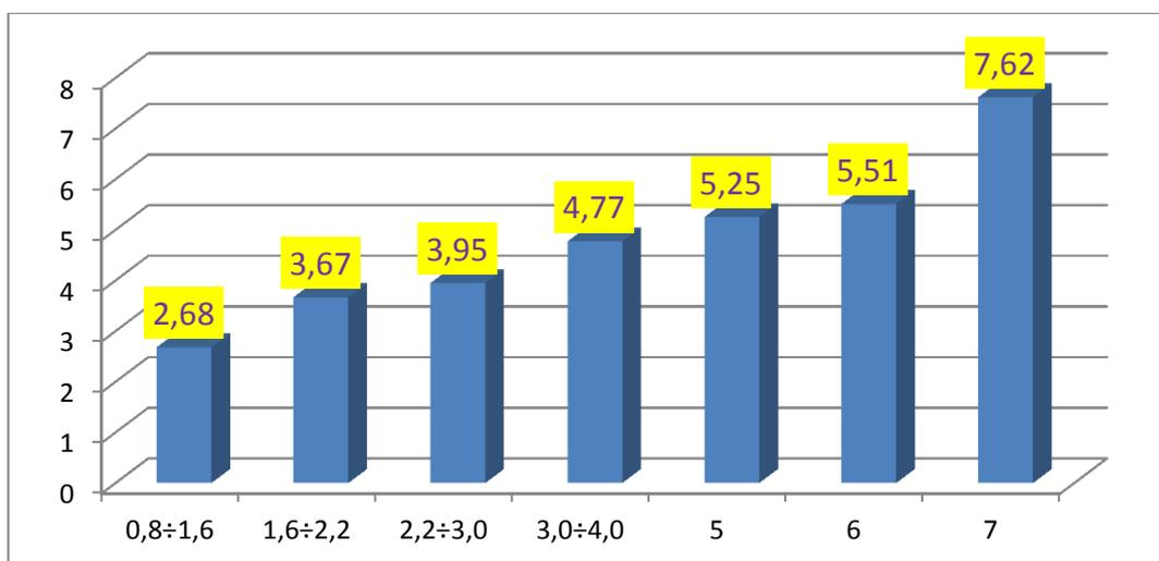
Fig. 2. Change in the relationship between the bulk density of expanded vermiculite and the coefficient of swelling of vermiculite concentrate
