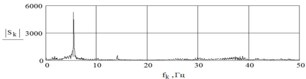
Fig. 6. Spectrum of vertical movements of a 27-meter metal beam, geophone №1, maximum spectral surge at a frequency of 5.52 Hz
