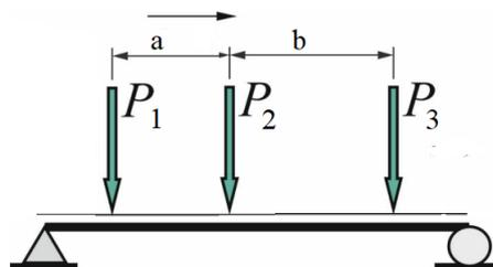
Fig. 1. Load model in the form of sequentially moving forces
