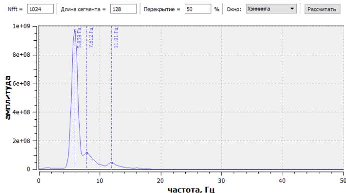
Fig. 11. Vibration frequency spectrum of superstructure No. 3 (left)
