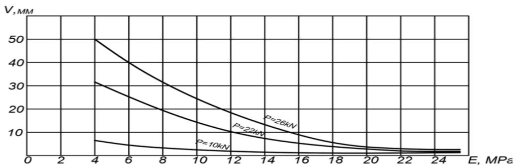
Fig.3. The effect of changes in the modulus of deformation of the soil and the degree of applied forces on the horizontal movements of the pile head.
