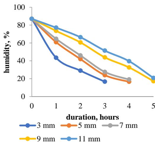
Fig. 6. Curves for combined infrared and convective drying at temperature 60°C of control samples of apple slices
