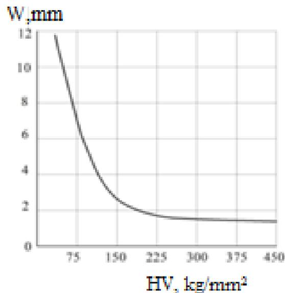
Fig.1. Effect of hardness on abrasive wear intensity [8]
