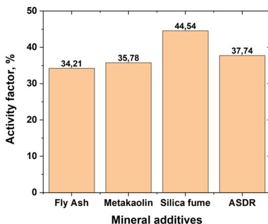
Fig.5. Activity coefficient of mineral additives
