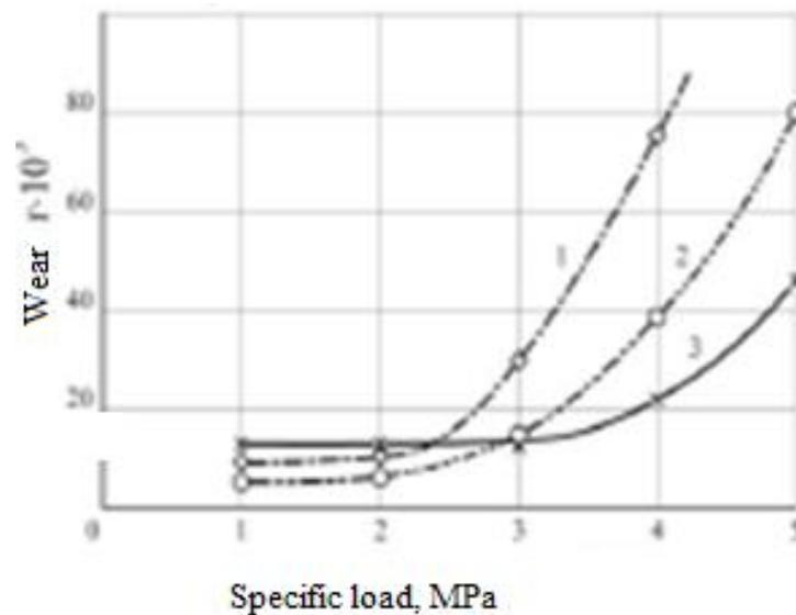
Fig.3. Effect of carbonitriding temperature on steel wear resistance (1 - 550°C; 2- 650°C; 3 - 750°C)
