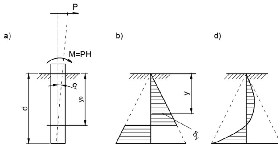
Fig.1. Soil pressure diagrams on the lateral surface of the foundation of the contact network supports under the action of horizontal load: a) scheme of load action on the foundation, b) soil pressure diagram in the limit state, c) the same in the elastic stage.
