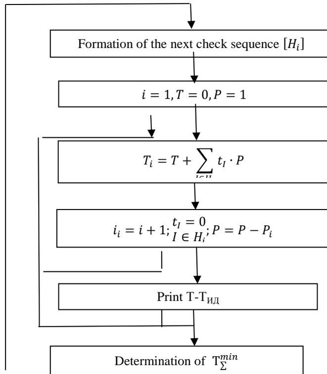
Fig.3. Algorithm for minimizing the loss during fault finding
