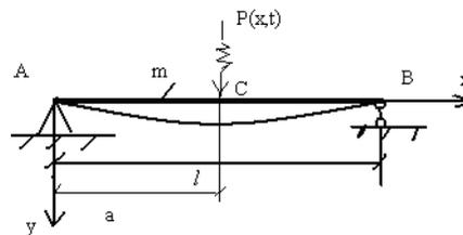
Fig. 2. Calculation scheme of forced vibrations of beam superstructures
