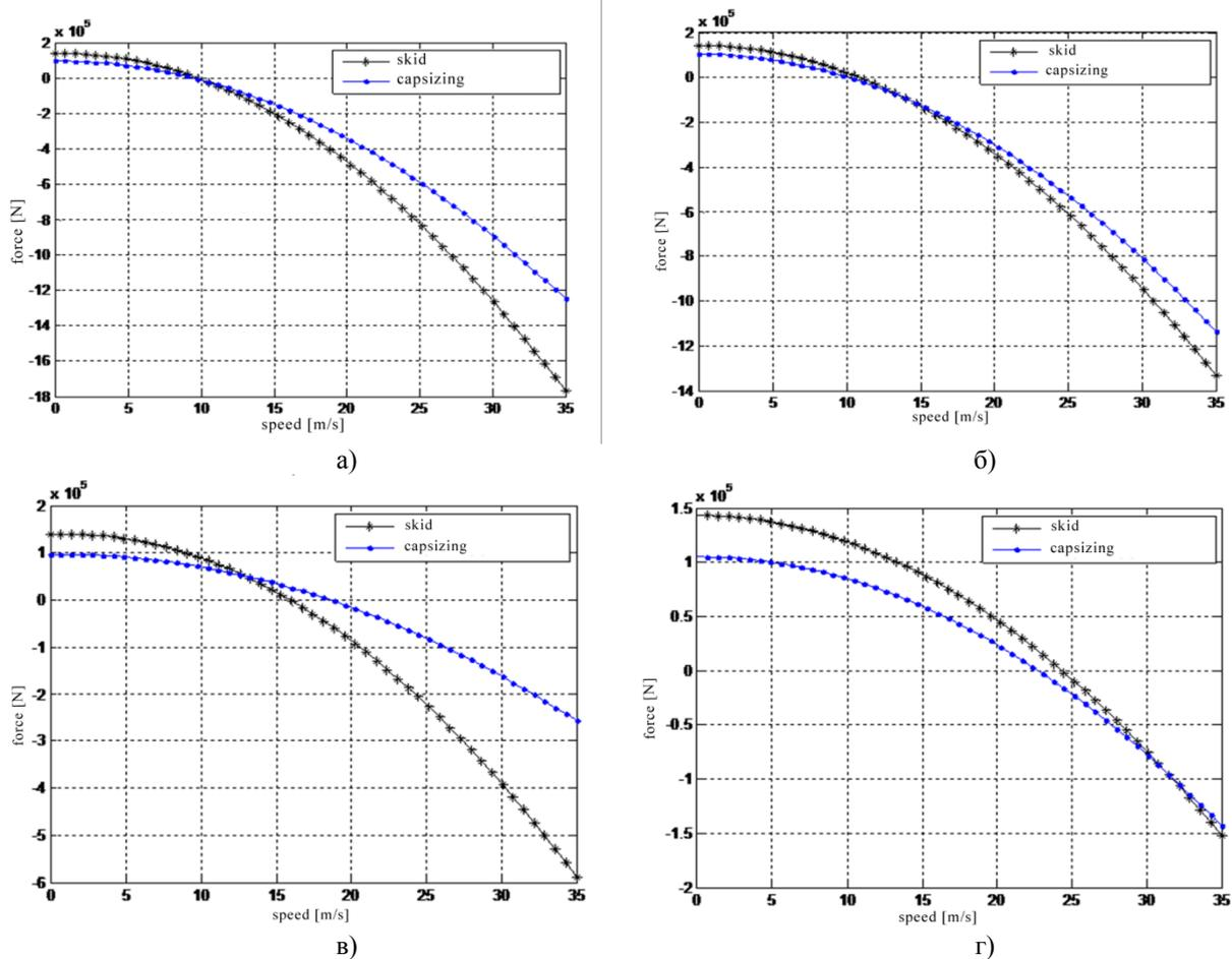
Fig. 2 The total impact of forces promoting and preventing rollover and skidding from the speed of movement of a semi-trailer train at different turning radii and longitudinal slope: a) taking into account, b) without taking into account the dynamic effect of the fluid at  $R=50 \text{ m}$ ,  $\alpha=3\%$ ; v) taking into account, d) without taking into account the dynamic effect of the liquid at  $R=200 \text{ m}$ ,  $\alpha=7\%$ ;
