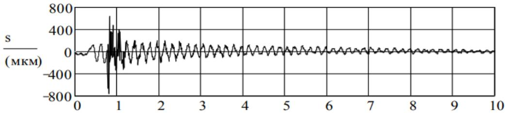
Fig. 3. Oscillogram of vibration displacement of the span structure of a metal bridge, seismic receiver №1
