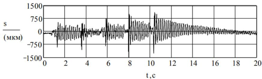
Fig. 5. Graph of vertical displacements of a 27-meter metal beam, geophone №1
