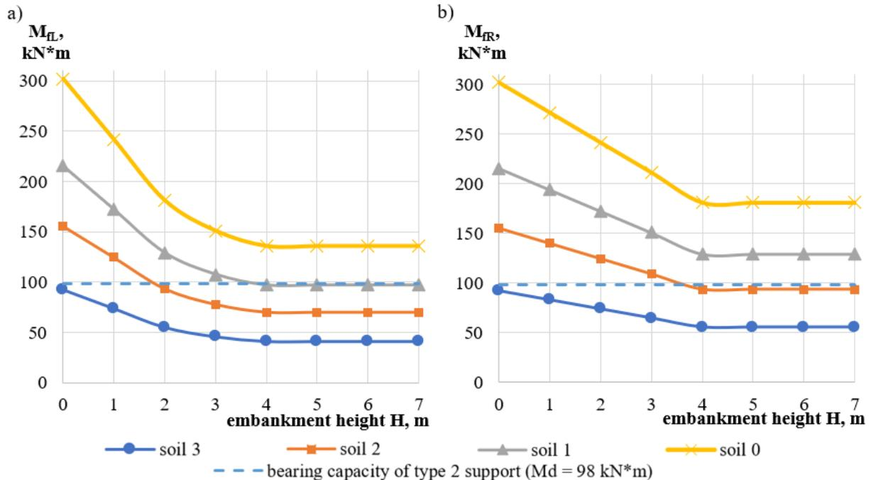
Fig.2. Graph of the change in the load-bearing capacity of the foundation on the action of the moment for different soils
