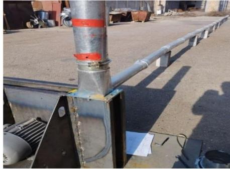
Fig. 1. Pneumatic transport with a 26 m pipe system
