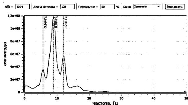
Fig. 7. Vibration frequency spectrum of superstructure No. 2
