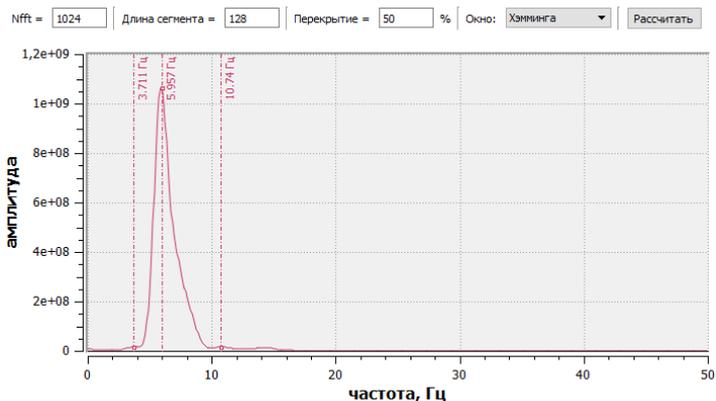
Fig. 10. Vibration frequency spectrum of superstructure No. 2 (left)
