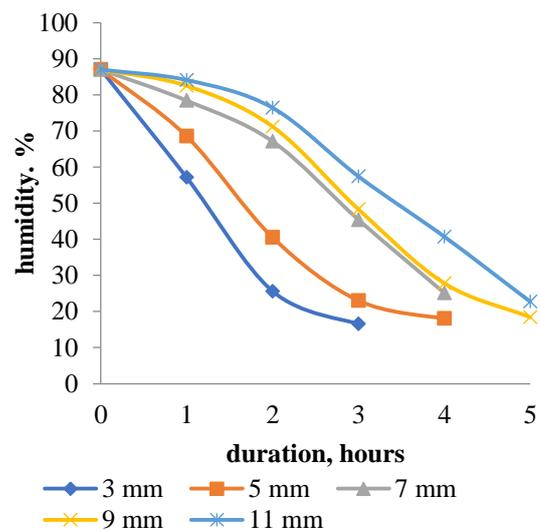
Fig. 3. Curves for combined infrared and convective drying at temperature 55 °C of apple slices treated by citric acid solution
