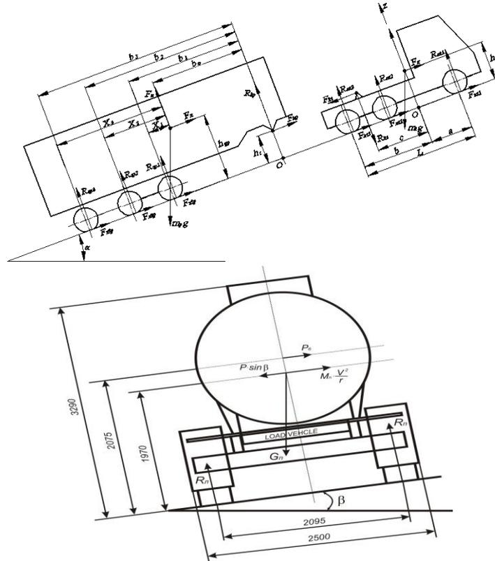
Fig. 1. Diagram of forces acting on a semi-trailer train when moving
