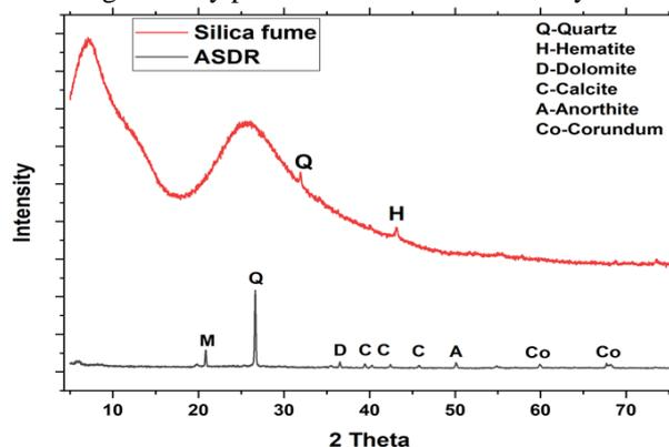
Fig.2. X-ray patterns of silica fume and slag ash mixture of dry disposal
