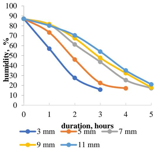
Fig. 4. Curves for combined infrared and convective drying at temperature 55 °C of apple slices treated by ascorbic acid solution
