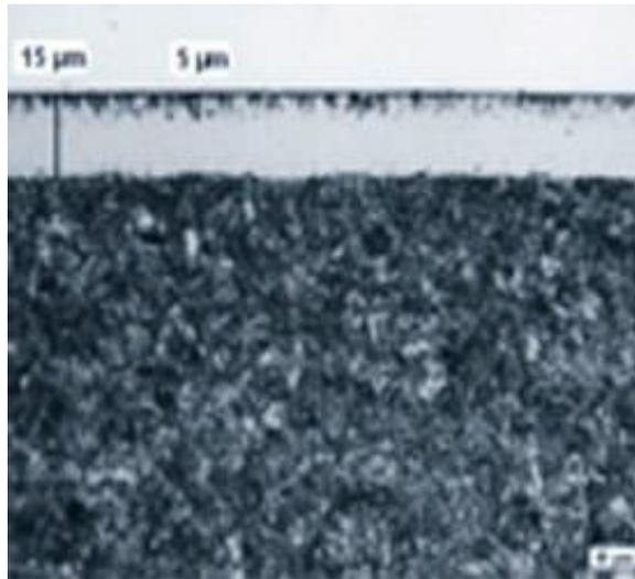
Fig.7. Structure and depth of the hardened layer [4]
