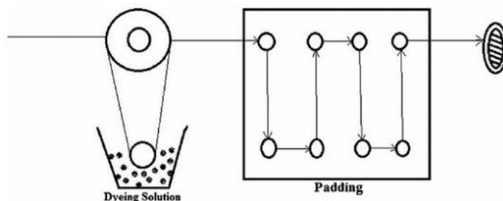
Fig. 3. Pad batch dyeing.
