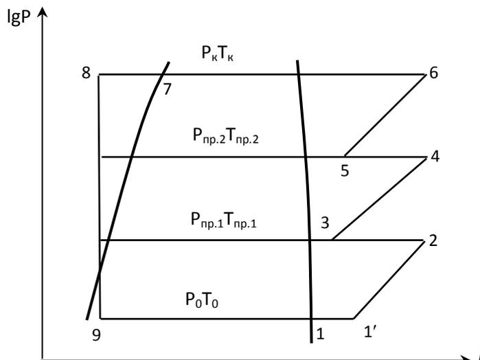
Fig. 1. Image of three-stage cycle processes heat pump (HP)  $\lg P - i$  in the diagram
