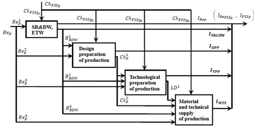
Fig. 4. Structural scheme of design and development processes interaction for the production with the technical purpose:
