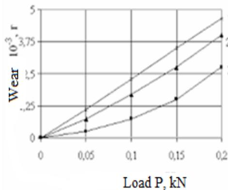
1 - steel 45 after improvement; 2 - steel 45 after carbonitriding; 3 – 38X2MIOA steel after improvement
