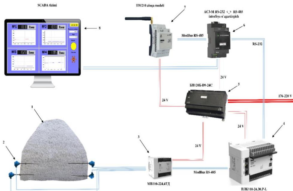
Fig 1. The scheme of measuring the temperature of one cotton bunt based on the SCADA system.
