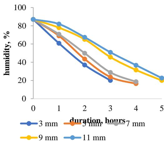
Fig. 8. Curves for combined infrared and convective drying at temperature 60 °C of apple slices treated by ascorbic acid solution
