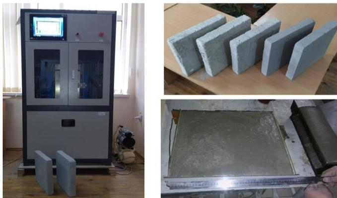
Fig 2. Equipment XND-2-3030C flat thermal conductor and prepared test samples.
