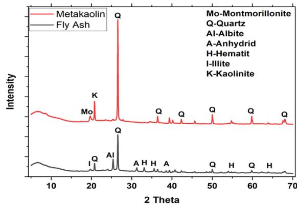
Fig. 1. X-ray patterns of metakaolin and fly ash
