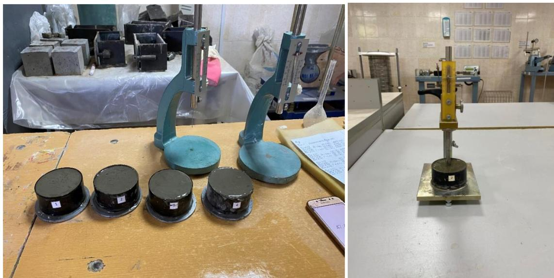
Fig. 1. Test samples on the Vica device
