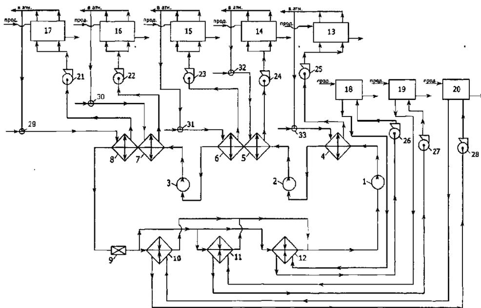
Fig. 2. Diagram of a heat pump drying unit with a three-stage compressor
