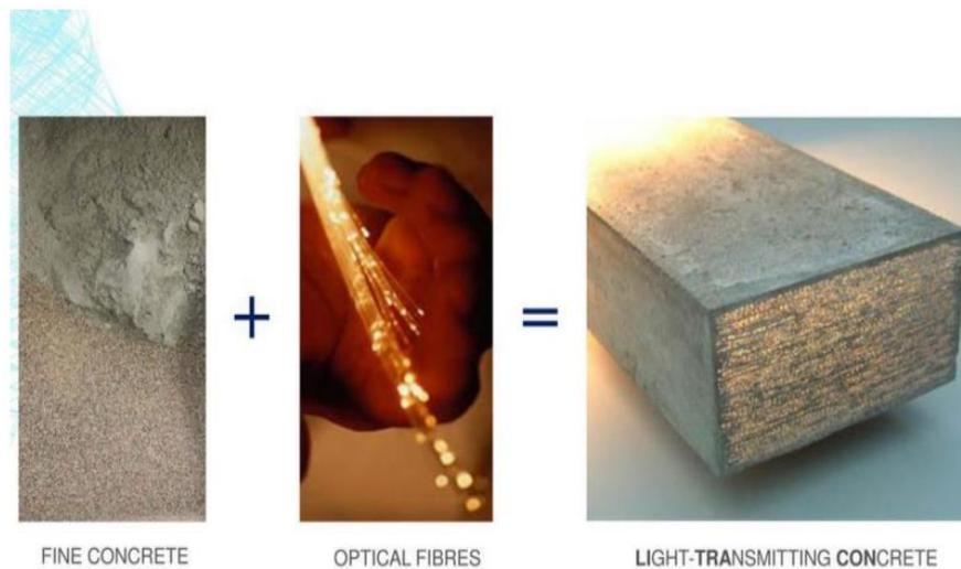
Fig.1. Materials and manufacturing process : a) fine concrete b) optical fibres c) light -transmitting concrete[3].
