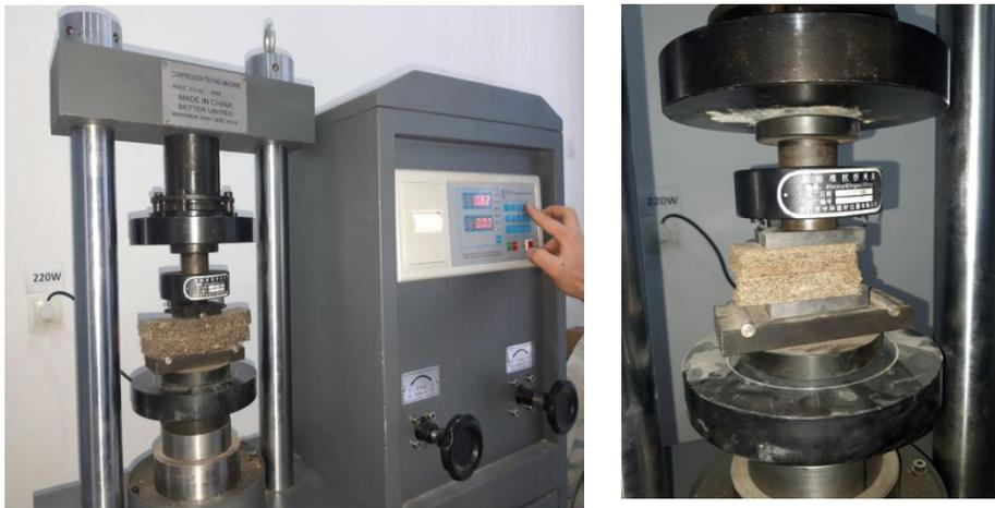
Fig.1. Determination of the strength of the vermiculite plate for bending and compression by experimental tests.
