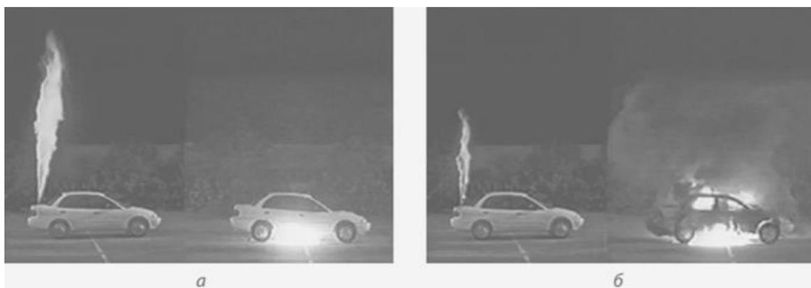
Figure 1. Experiment to check the consequences of depressurization of the fuel tank of hydrogen (a) and gasoline (b) cars
