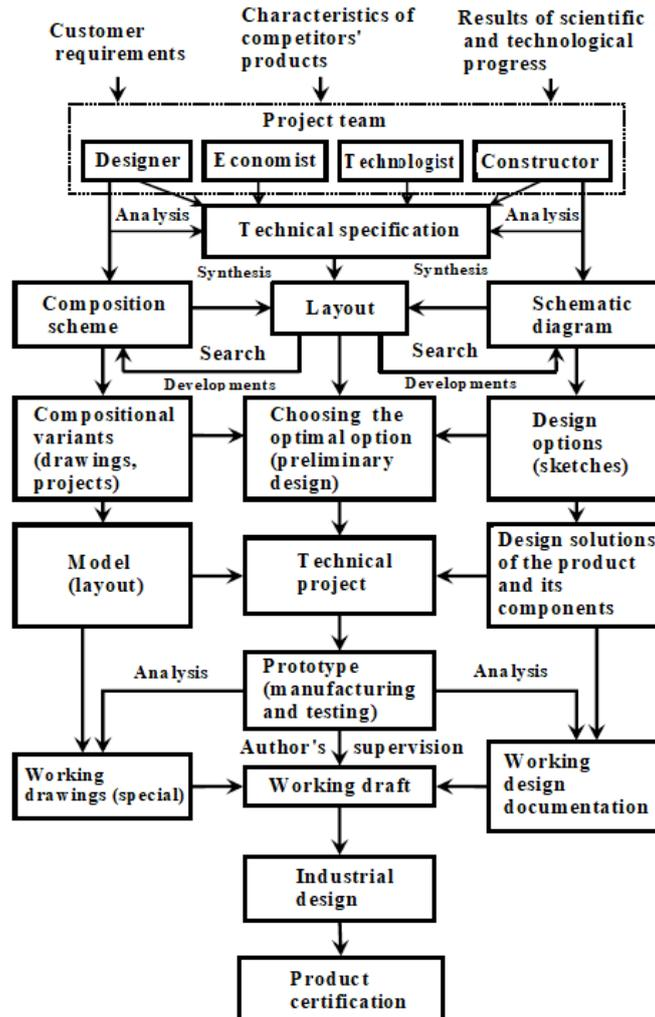
Fig. 2. Structural scheme of works at development of technical project
