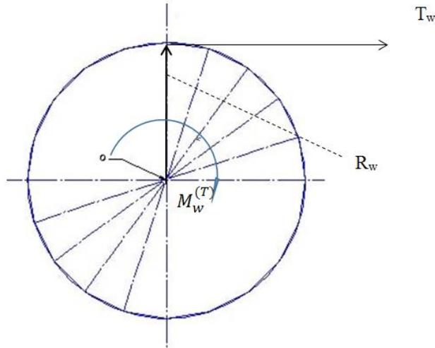
Fig. 1. Direction of torque and tension force in wheel rotation
