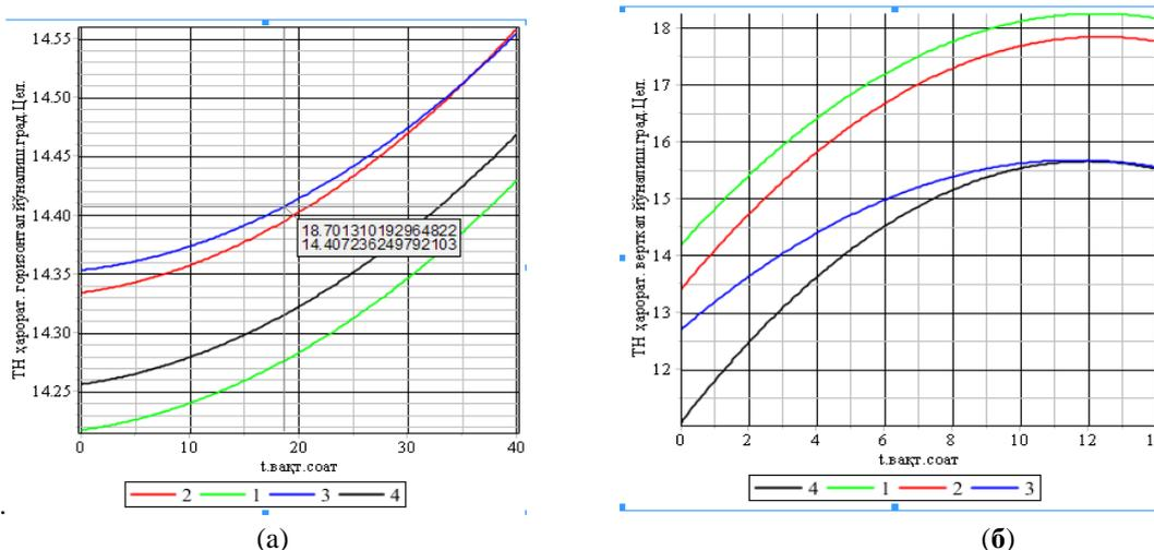
Table 2. The regularity of changes in the temperature of raw cotton in the horizontal (a) and vertical (b) directions.
