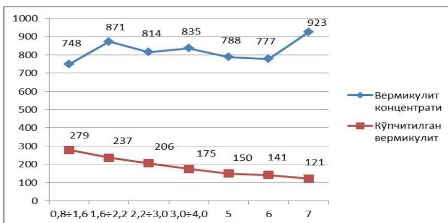
Fig. 1. Change in the relationship in the grain section between the bulk density of vermiculite concentrate and expanded vermiculite
