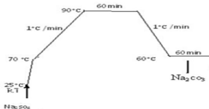
Fig.1. Dyeing process of cotton polyester fabric with chitosan
