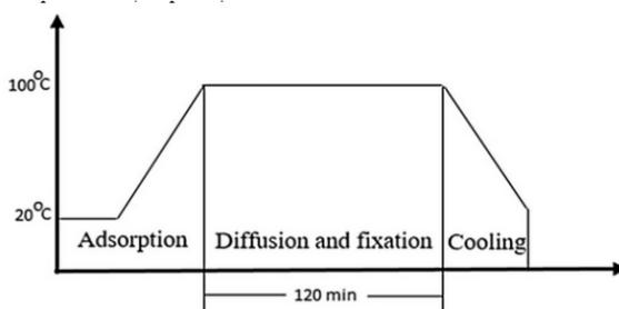
Fig. 1. Line diagram of exhaust dyeing
