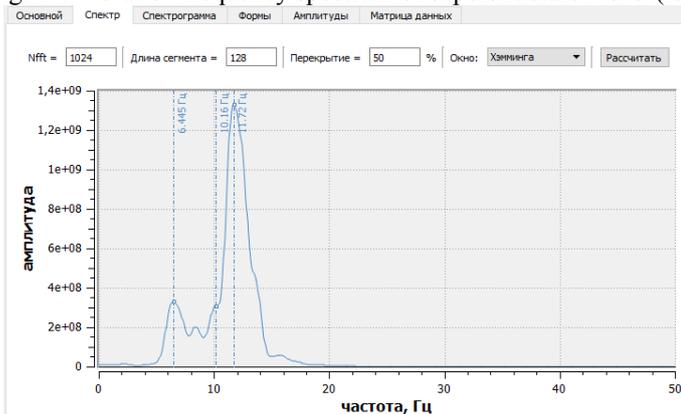
Fig.12. Vibration frequency spectrum of superstructure No. 4 (left)
