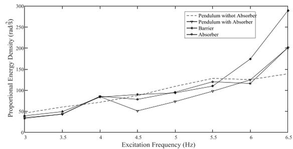
Fig.5. Comparison of the proportional energy density of the proposed mechanism with the simple pendulum
