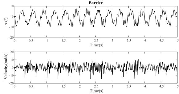
Fig.3. Time response of the barrier velocity and displacement
