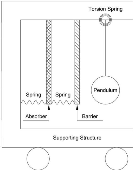
Fig.1. Mechanical frequency up-conversion mechanism
