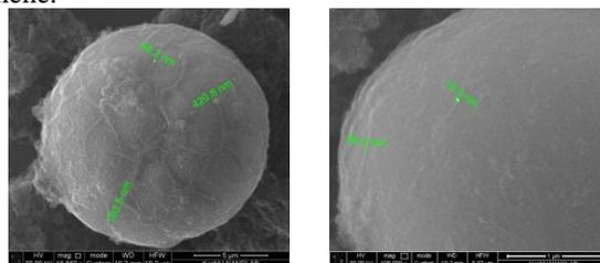
Fig. 1 Micrographs of microstructures of nickel particles in a carbon shell
