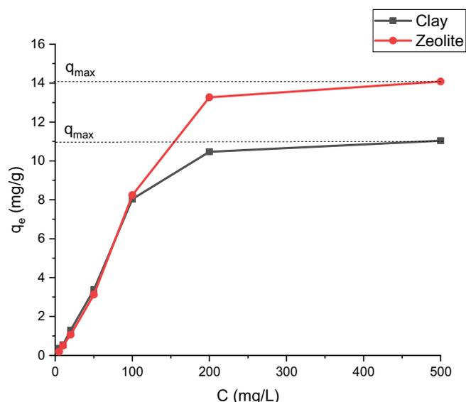
Fig. 2. Pb $^{2+}$  ions adsorption isotherm on the natural zeolite and Chamotte clay.
