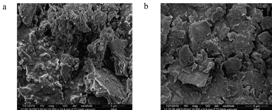
Fig. 1. SEM-image of (a) natural zeolite; (b) chamotte clay.
