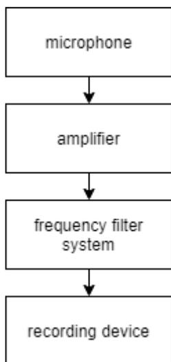
Fig. 2. Block diagram of a phonocardiograph
