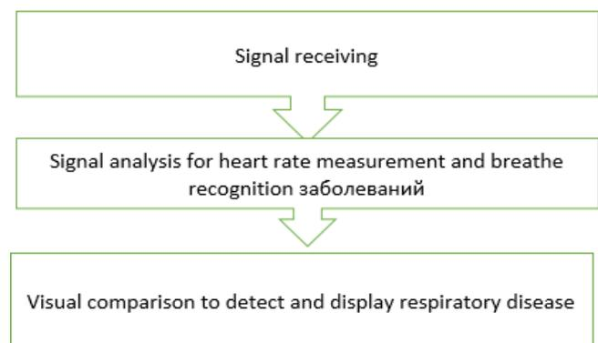
Fig. 3. Working principle of the smart stethoscope
