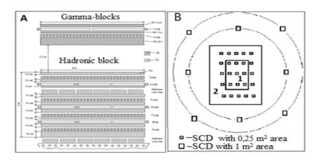
**Fig.1.** A – ionization calorimeter, composed of gamma-blocks and lower on 2,2 m hadronic block. B –installation detectors disposition circuit (top view): 1-calorimeter disposition in the laboratory housing. 2- SCD by 0.25 m<sup>2</sup> area disposition in the laboratory housing. In the closest circle within a radius of 40 m and in large circle within a radius of 100 m in fours SCD with 1 m<sup>2</sup> area are disposed.
