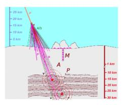
**Fig. 3.** Model of deeper seismic sounding of Earth's crust on the basis of muons from the energetic EAS trunk: P is a deep fault zone; A is elastic vibrations are generated in the seismic stretch environment under local ionization influence from muons passing and propagated as acoustic wave; M is a sensible microphones system.
