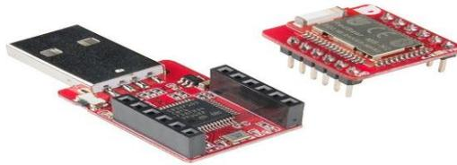
Figure 1. BLE Nano kit microcontroller
