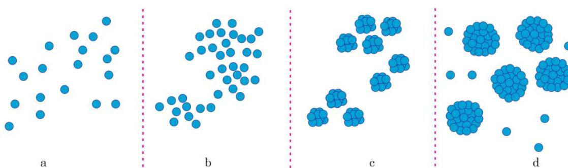
Fig. 2 – Mechanism of growth of nanoparticles in RF plasma: nucleation phase (a), saturation phase (b), coagulation phase (c), surface growth phase (d)
