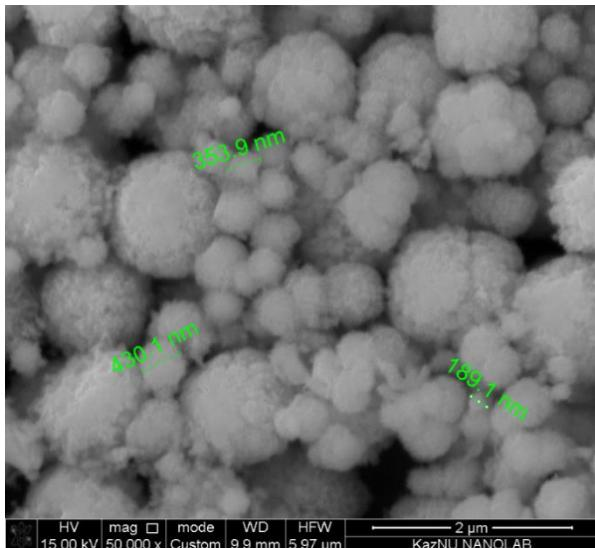
**Fig. 5 – SEM image of copper nanopowder**
