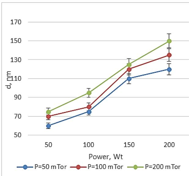
**Fig. 7 – Dependence of the diameter of synthesized particles on the power of discharge**
