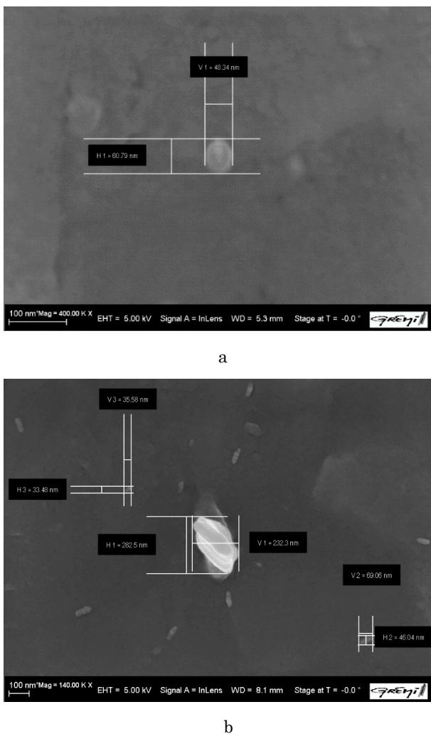
**Fig. 3 – SEM images of copper nanoparticles: power 100 W (a), 150 W (b)**
