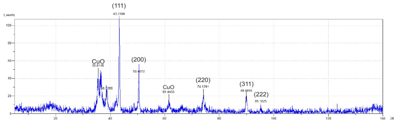
**Fig. 9 – XRD pattern of copper nanopowders**
