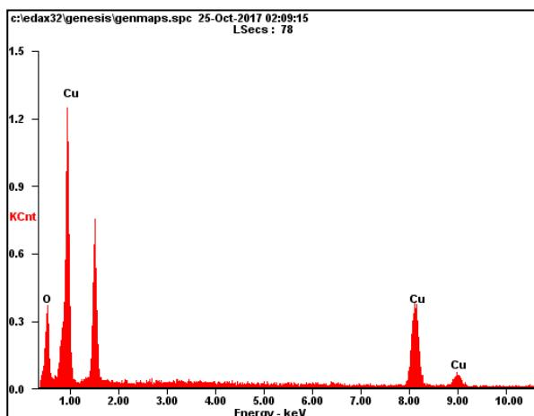
**Fig. 6 – The energy dispersive spectrum of copper nanopowders**
