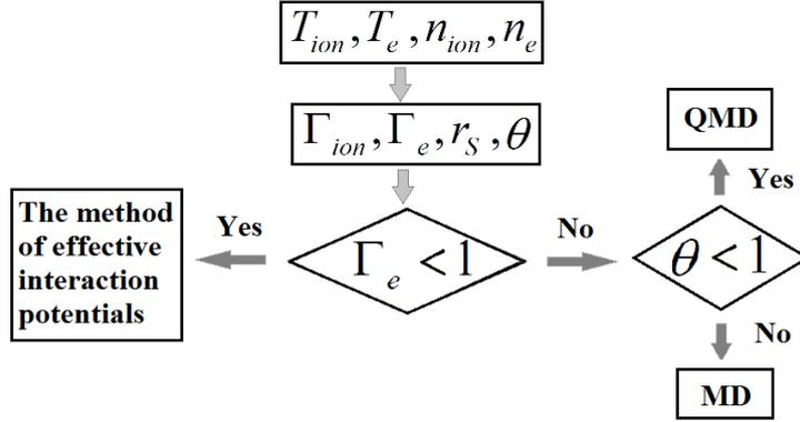
**Figure 1.** The diagram shows the case when the effective interaction potentials can be used for straightforward calculation of the scattering cross sections and transport properties of the plasma. In the case of plasma with non-ideal electrons molecular dynamics simulation (classical or quantum) of two component plasma should must in order to determine dynamical properties of plasma.
