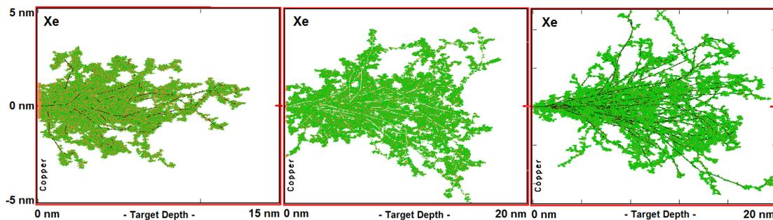
**Figure 3.** Results obtained from SRIM: The trajectories of the xenon ions in the copper with an initial energy of 5 (on the left), 15 (in the middle) and 30 keV (on the right).
