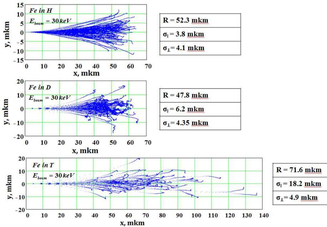
**Figure 1.** The trajectories of iron ions with an initial energy of 30 keV hydrogen isotopes: (from the top) protium, (in the middle) deuterium and (from the bottom) tritium. The figure also shows the stopping range and the dispersion in the longitudinal and transverse directions.
