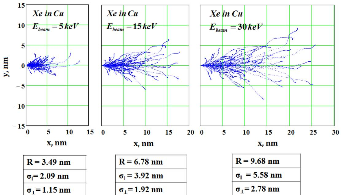
**Figure 2.** The trajectories of the xenon ions in the copper with an initial energy of (from the left) 5, (in the middle) 15 and (from the right) 30 keV. Figure shows the stopping range of the xenon ions depending on the energy in copper.
