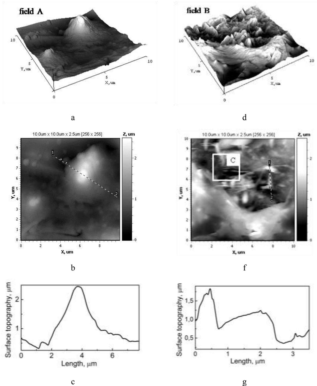
**Figure 3.** 3D- and 2D maps of the surface and cross section profile between markers 1 and 2 for site A (a, b, c) and site B (d, f, g) of coating Fe-Co-Mo. Scan area AFM 10.0 $\times$ 10.0 $\mu\text{m}$ . Thickness is 8 $\mu\text{m}$ .
