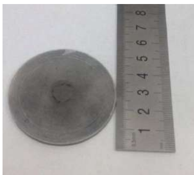
Figure 1 - Solid oxide target for pulsed laser deposition
