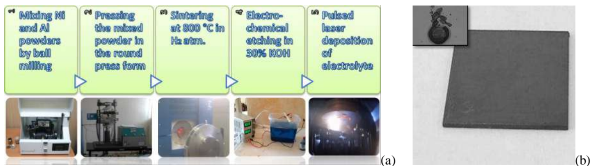
Figure 2. a) Schematic diagram for the porous nickel anode fabrication process, b) The fabricated porous nickel anode 10x10 mm.
