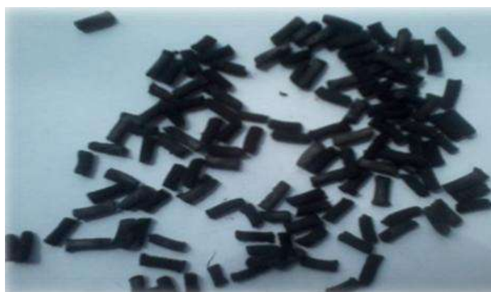
Figure 2 - Granular carbon sorbent from RH and lignosulfonate
