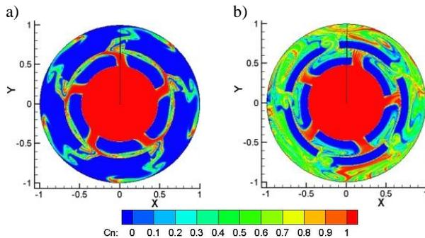
Figure 3: Dynamics of changes in concentration of the hydrocarbon blend's components at angular speed  $\omega_1 = 314$  rad/s revolutions per second at a time a)  $t = 0.25$ , b)  $t = 1.5$
