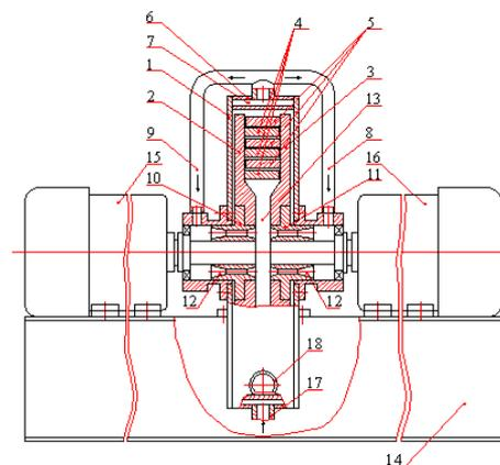
Figure 1: Diagram of the pilot version of the hydrodynamic activator.
