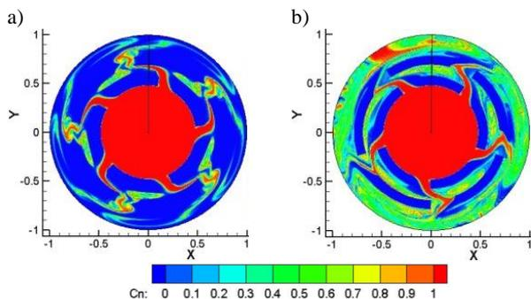
Figure 4: Dynamics of changes in concentration of the hydrocarbon blend's components at angular speed  $\omega_2 = 377$  rad/s revolutions per second at a time a)  $t = 0.25$ , b)  $t = 1.5$
