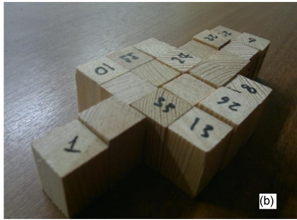
Fig. 1. Larch pieces: (a) bending test peice; (b) pressure test pieces
