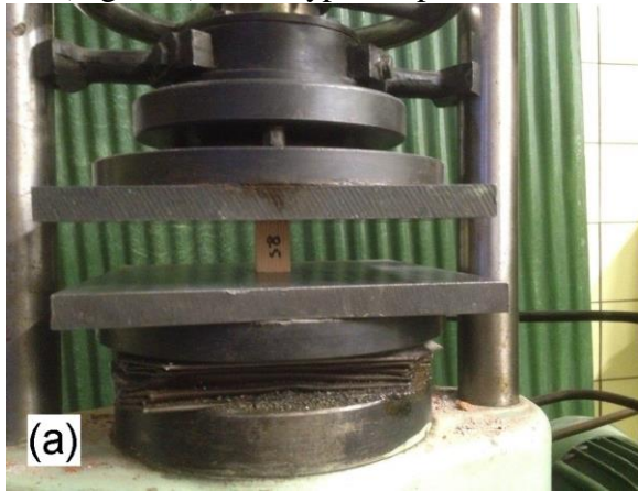
Fig. 2. Test operation: (a) pressure along grains; (b) static bending
