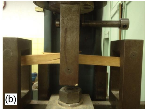
Fig. 2. Test operation: (a) pressure along grains; (b) static bending
