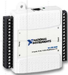
Figure 4: DAQ card NI USB-6008
