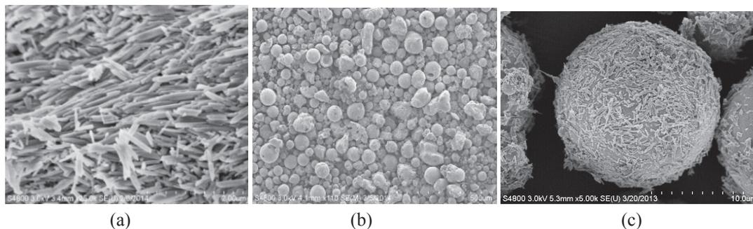
Fig 1. SEM images of a) halloysite nanotubes, b) fly ash particles, and c) fly ash particles surface coated with polyelectrolytes followed by mixing with halloysite nanotubes.
