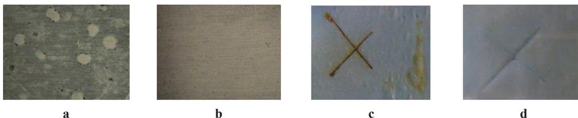
Fig. 1. Optical image of a corrosion process developed for 6 months in 0.5 M NaCl solution: on (a, b) aluminum coated by a 40  $\mu\text{m}$  thick layer of (a) conventional polyurethane paint and (b) the same paint doped with 5 wt % halloysite loaded with hydroxyquinoline and (c, d) a steel plate coated by (c) polyurethane paint with artificial scratches and (d) the same paint doped with 5 wt % halloysite loaded with dodecylamine.
