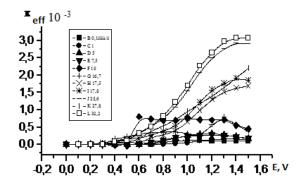
**Figure 3.** The dependence of the effectiveness coefficient of anodic dissolution of molybdenum on potential at the different concentrations of LiCl and  $0.5 \text{ M Mg}(\text{ClO}_4)_2$ .
