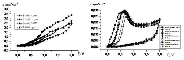
**Figure 1.** The polarization curves of the anodic dissolution of molybdenum in 0.25 M LiCl in DMSO.
