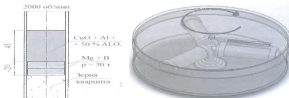
Fig. 3 – The load scheme of initial mixture in reactor of the high temperature centrifuge and main body of centrifuge
