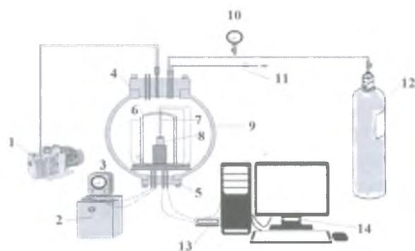
1 - the vacuum pump 2 - transformer, 3 - ampermeter 4 - upper cover of the reactor, 5 - the bottom of the reactor lid 6 - tubular heating furnace 7 - thermocouple 8 - sample 9 - reactor vessel 10 - manometer 11 - intake and exhaust valves 12 - nitrogen cylinder 13 - collection system data LTR-U-1 14 - a computer
